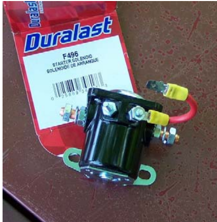
Here's how the wires attach to it.
